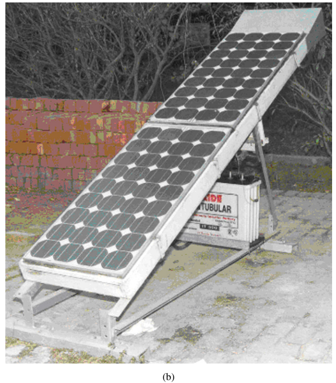
Fig. 1. (a) Schematic diagram of hybrid PV/T air collector. (b) Photograph of experimental setup of hybrid PV/T air collector at IIT Delhi.
